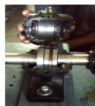
Cap off, old grease out, fresh grease in — before the first start after long storage.
